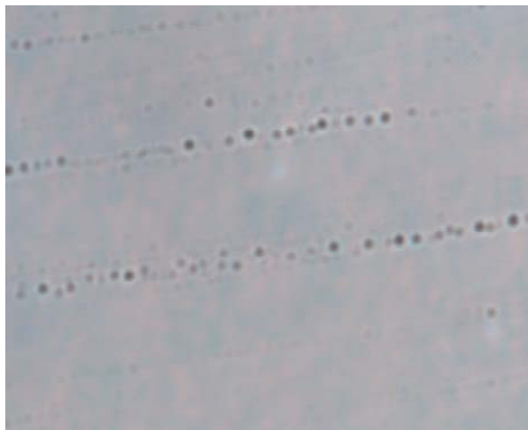
Fig. 8 Microscopic view of biofilm samples in cast iron coupons in AR2 for 168 days with mono chloramine disinfectant.
