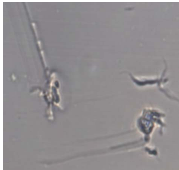
Fig. 9 Microscopic view of biofilm samples in cast iron coupons in AR2 for 158 days with mono chloramine disinfectant
